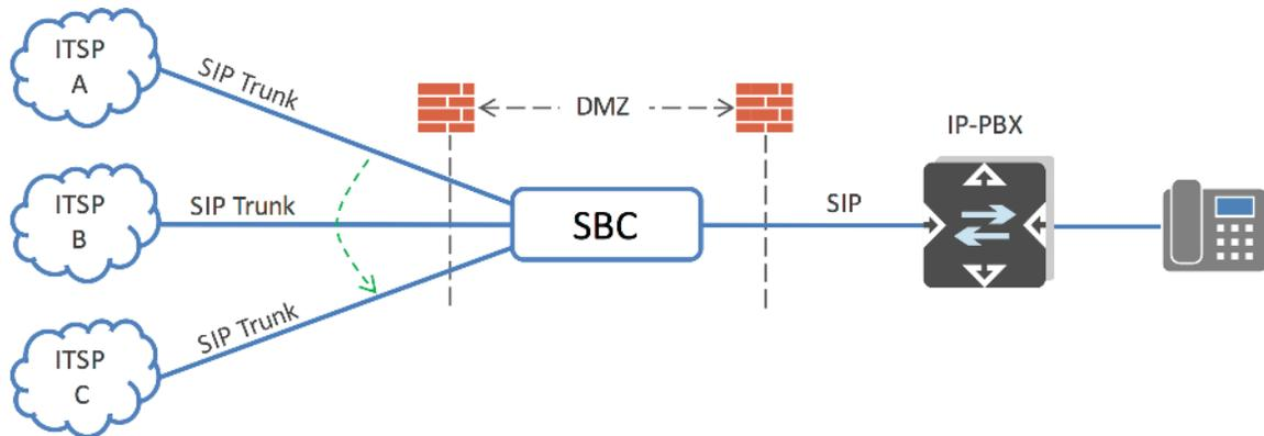
SBC protects VoIP network and provides load balancing across SIP trunks
