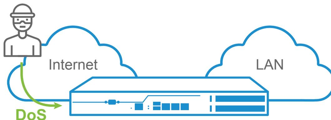
The SBC is designed to protect mission critical Unified Communications (UC) applications such as IP PBXs, IVR, call centers, and more. The SBC contains features, such as Intrusion Detection System (IDS) and Intrusion Prevention System (IPS), specifically designed for SIP applications, detecting attacks and automatically adjusting to prevent the DoS attack from traversing into the private network.
