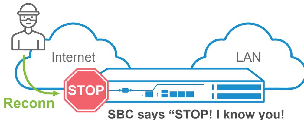
The SBC is designed to do just that. It recognizes these SIP scanners by their 'signature' and rejects them. Not responding to SIP scanners allows the VoIP deployment to be hidden from future security attack attempts, making it harder for malicious parties to compromise your network.
