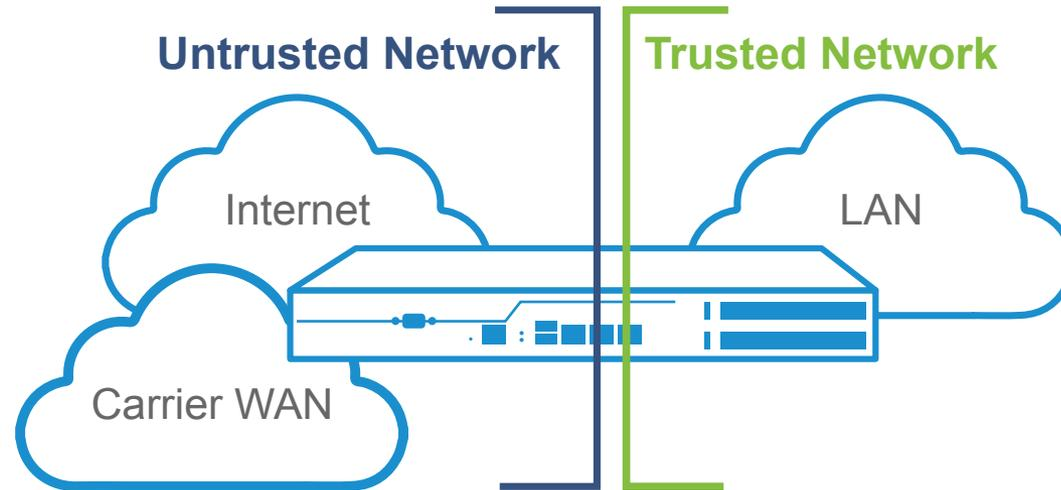
Every VoIP device in the call flow path is responsible to prevent toll fraud, but the SBC may be the most important. Tools built into the SBC, such as rate limiting, blacklisting, and advance call control, help identify potential toll fraud activities. Other features, such as SNMP and SMTP alert notifications, alert IT administrators to potential issues. Simply put, the SBC is designed to play an integral role in toll fraud prevention.
