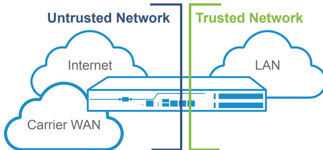
It is important to place an SBC between trusted and untrusted IP networks to provide security policies and ensure that each network does not have a direct connection. The Internet is the most untrusted IP network, and even private WAN IP networks should be considered untrusted for the security of the enterprise trusted LAN network.
