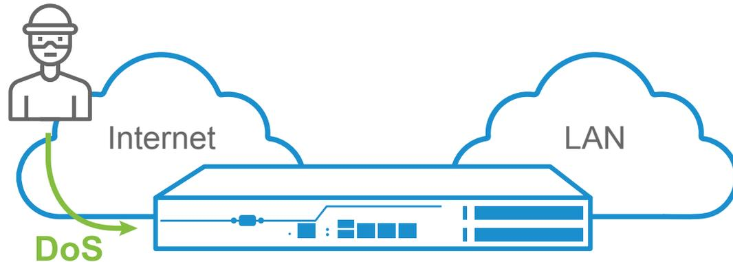
The method for Rate Limiting on SIP is to determine the number of INVITEs or new calls that the SBC is going to allow to traverse through to the VoIP servers. This is beneficial when wanting to restrict the number of new calls presented in a given period of time.
